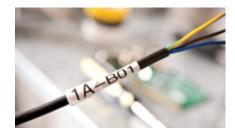
Heat-shrink tube Shrinks and grips cable when heat is applied.
