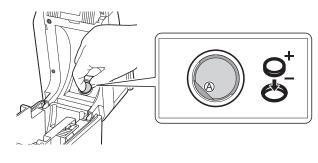
5 Return the time/date battery cover to its original position, and then use a coin or similar object to slowly turn the time/date battery cover in the opposite direction of the arrow on the battery cover until it stops in order to install the time/date battery cover.
