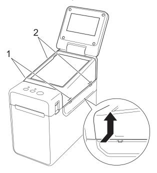
2 Remove the TDU panel cover, and place the touch panel (1) to be used, then the clear protective sheet (2) on the touch panel holder (3).
